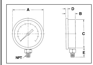
CASE & RING: 4" type 304 stainless steel case with polished stainless steel crimped ring. DIAL: White aluminum with black and red markings. (psi&Kpa) WINDOW: Clear acrylic. TUBE: Phosphor Bronze. SOCKET: Brass with threaded restrictor. POINTER: Black anodized aluminum. MOVEMENT: Brass rotary type with bushings. ACCURACY: 1% of span. ANSI B40.1 Grade A CONNECTION: 1/4" NPT bottom. RANGES: Vacuum, Compound, Pressure to 1000 psi.
