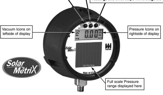
**Resolution-** The Weiss SolarMetriX® pressure gauge includes automatic rounding to standard increments. The first half of the range has display resolution of approximately 1/4% and the upper half of the range rounds to approximately 1/2% of the full scale.
