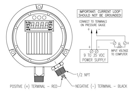
VOLTAGE/PRESSURE EXAMPLE FOR 200PSI  $R_L=250\Omega$
